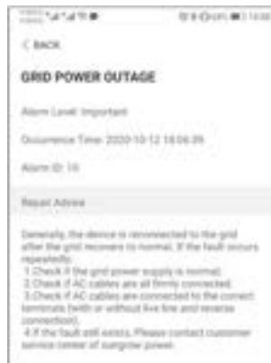
figure 7-9 Detailed Fault Alarm Information
