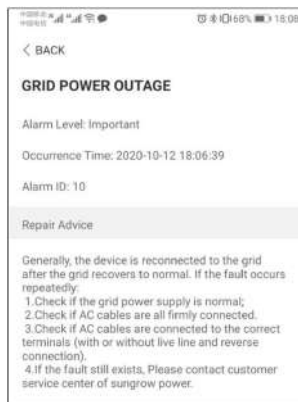
figure 7-9 Detailed Fault Alarm Information
