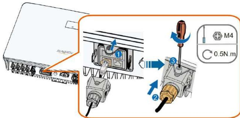
**step 6** Slightly pull out the cable and then fasten the swivel nut. Lock the connector with the screw.
