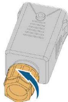
**step 3** Thread the BACKUP cable through the swivel nut, appropriate sealing and waterproof cover in sequence.
