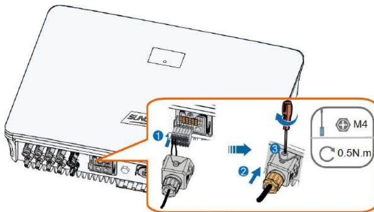
**step 8** Slightly pull out the cable and then fasten the swivel nut. Lock the connector with the screw.
