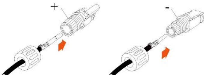
**step 4** Check for polarity correctness.
