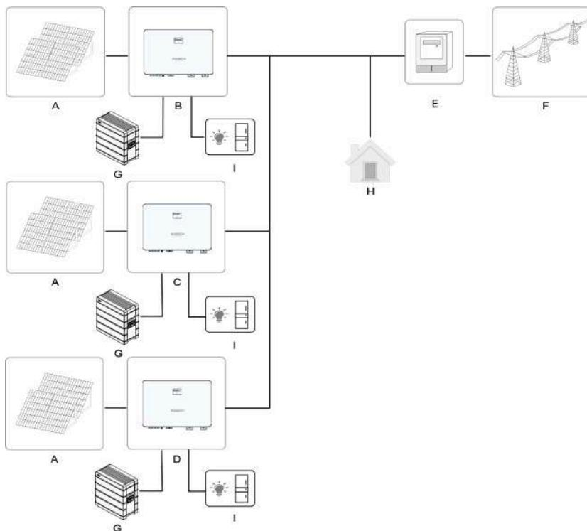
**figure 2-5 Grid-connected Parallel System (With Backup Load)**
