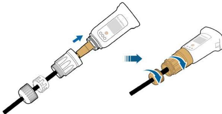
**step 6** Remove the waterproof lid from the terminal and install WiNet-S2.
