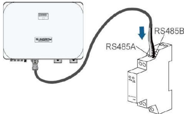
**step 11 (Optional)** If the length of the communication cable > 10m, please connect a 120Ω resistor in parallel to the meter. Plug the resistor directly into both RS485 communication ports.
