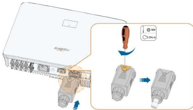
**step 2** Before connecting the emergency load to the Backup terminal, unscrew the swivel nut and take out the sealing ring first.
