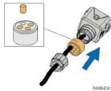
**step 5** Plug the wires into the corresponding terminals as shown in the following figure. Ensure that the wires are securely in place by slightly pulling them.
