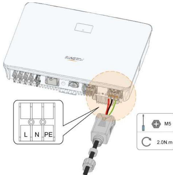
**step 8** Secure the AC waterproof cover to the inverter with a torque of 0.5 N•m and tighten the swivel nut to a torque of 5 N•m–6 N•m.
