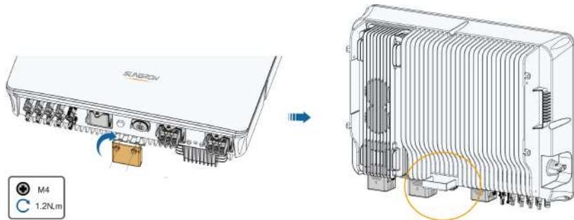
**step 4** Lift the inverter and slide it down along the wall-mounting bracket to make sure they match perfectly. Use two screw sets to lock both left and right sides.
