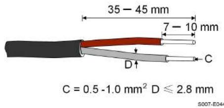
**step 2 (Optional)** When using a multi-strand wire cable, connect the wire head to the cord end terminal.
