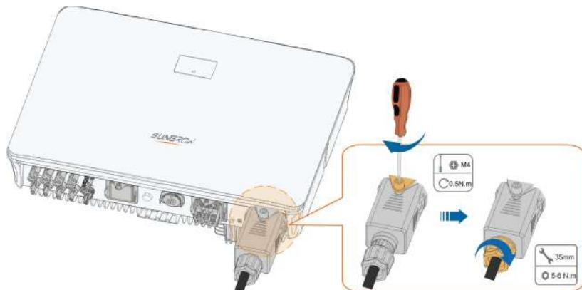
**step 9** Connect the PE wire to ground and the phase lines and the "N" line to AC circuit breaker. Then connect the AC circuit breaker to electric board.
