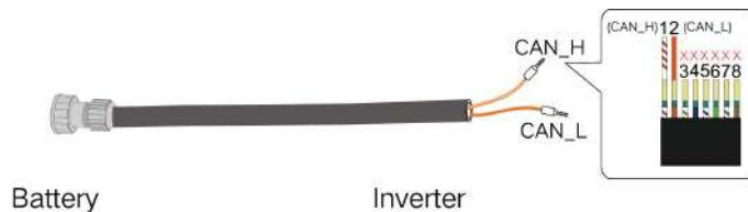
The battery communication cable is connected to the inverter COM2 ports H and L.
