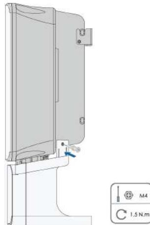
**step 5** The installation of the protective cover is completed.
