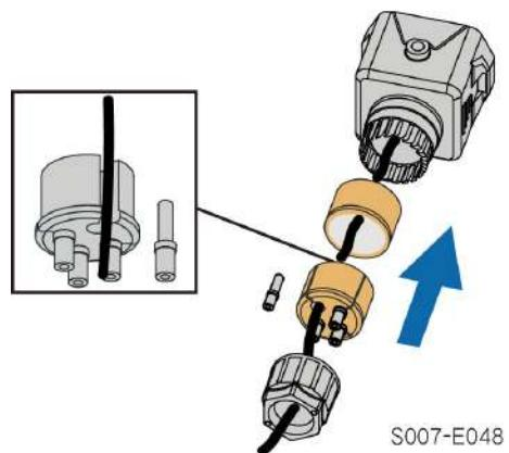
**step 5** Plug the wires into the corresponding terminals as shown in the following figure. Ensure that the wires are securely in place by slightly pulling them.
