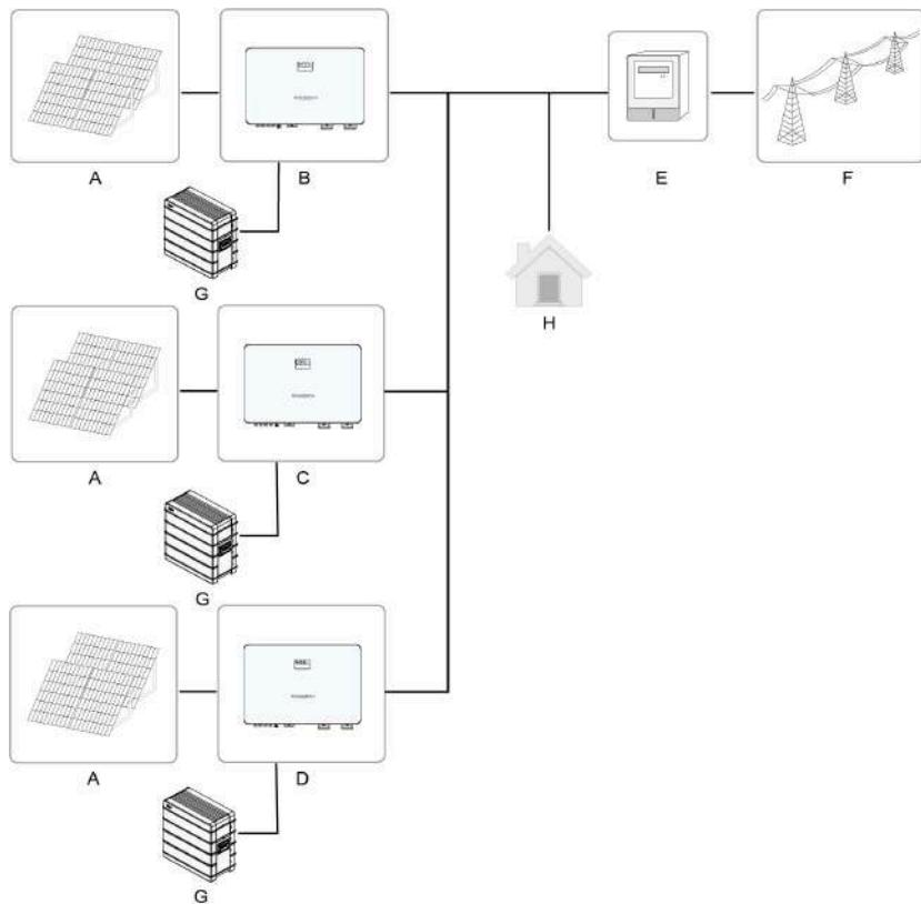
**figure 2-4** Grid-connected Parallel System (Without Backup Load)
