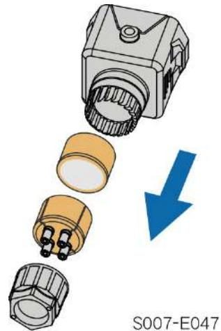
**step 4** Lead the cable through the cable gland.
