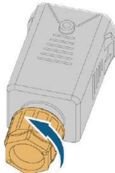
**step 3** Thread the AC cable through the swivel nut, appropriate sealing and waterproof cover in sequence.
