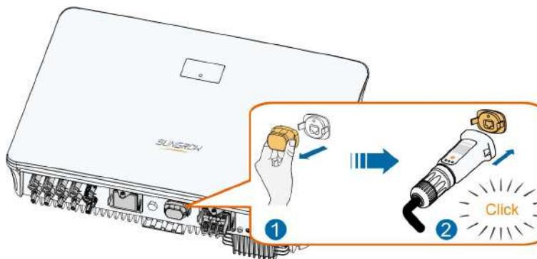
**step 7** Slightly shake it by hand to determine whether it is installed firmly.
