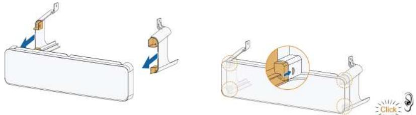
**step 3** After the electrical connection of the inverter is completed, install the protective cover to the inverter bottom and make sure that the threaded holes in buckles of the protective cover are aligned with the holes on the sides of the inverter.
