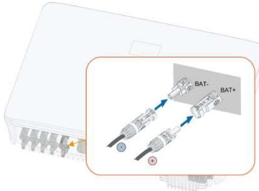
**step 7** Ensure that the connectors are securely in place.
