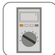
Multimeter ≥ 1000V DC
